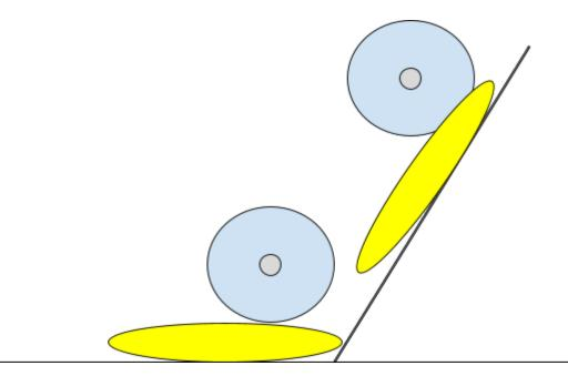
Our initial design of the disc collection system is quite simple. There is a ramp in the back with a pair of flex wheels spinning at high speed (200 RPM). The flex wheels will pick up the yellow discs from the floor and force them to move along the ramp to go upwards. The next pair of flex wheels will continue pushing the yellow discs further up until they reach the shooter disc holding area.
