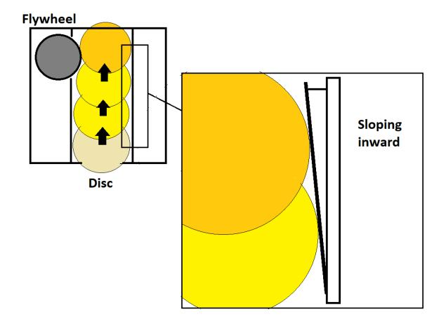
With this new design, we also tried using pneumatics. Previously, we did not use pneumatics and this put us at a major disadvantage as we could not have more mechanisms that would potentially help us. So, after seeing many other robots using pneumatics, we also decided to give it a try. We used pistons to push the disc up to where the flywheels would be for **2 main reasons**:
