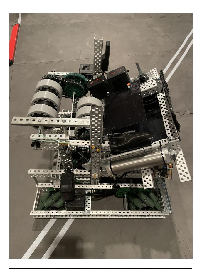
After much trouble shooting, we discovered that the collection flex wheels RPM is too low (200 RPM). After we switched to a high RPM (600 RPM), all the above problems went away. As it turned out, the discs don't have enough momentum to go all the way up the ramp. A faster flex wheels solved the problem.
