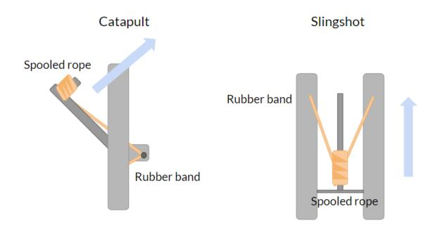
However, after testing, we saw that both of these designs could not launch the rope far enough and it just was not consistent enough. It was also extremely hard to set up. So, we decided to adopt the idea from our disc shooter trigger and used the sliding piece with a rubber band on it. We did this because we thought it would be easier to set up and slide easier.
