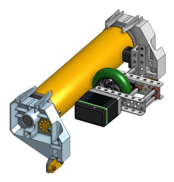
The design of the roller spinner is rather straight-forward. Basically, we already have spinning flex wheels that we use to collect discs from the floor. We just need to chain those flex wheels to a wheel that is at the right height to spin the roller.
